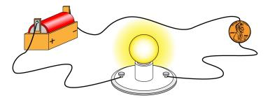
Touch the free ends of the wire to the object you are testing. If the light bulb lights up, the object is made from a conductor. if it does not, the object is made from an insulator.
