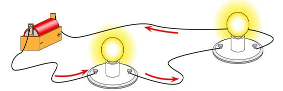
If a light bulb is missing or broken in a series circuit, will the other bulb light? Explain.
